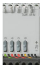
Local override, three-colored LEDs
