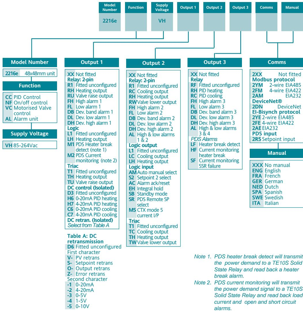
Note 1. PDS heater break detect will transmit the power demand to a TE10S Solid State Relay and read back a heater break alarm.
