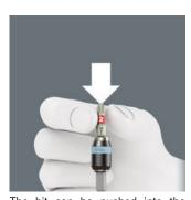
The bit can be pushed into the adaptor without moving the sleeve. The lock is activated automatically as soon as the bit is applied to the screw. Bits are held securely and wobble-free.
