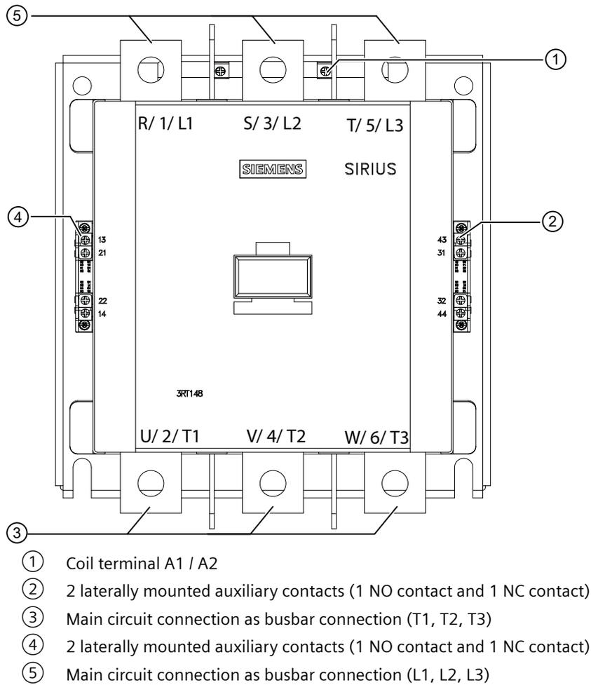
Figure 4-15 3RT1481 power contactor, overview (example illustration)
