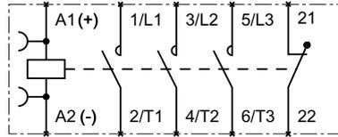
S00 contactor, without RC circuit, 1 NC contact
