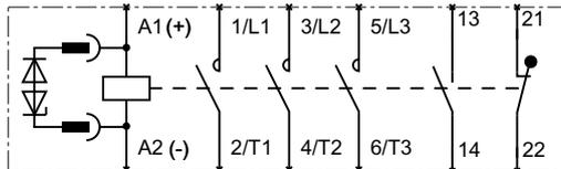
S0 contactor, with internal diode, 1 NO contact, 1 NC contact
