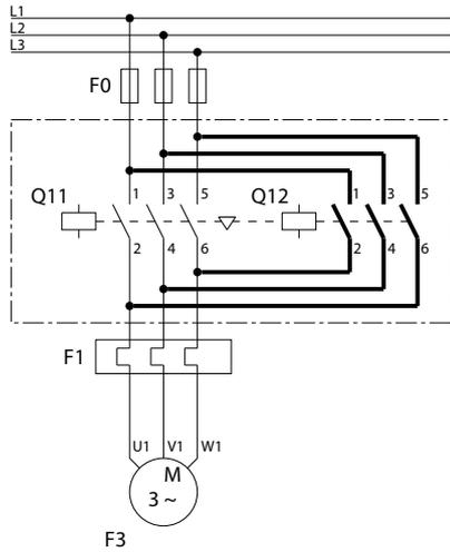
Figure 6-19 Main circuit of the reversing contactor assembly
