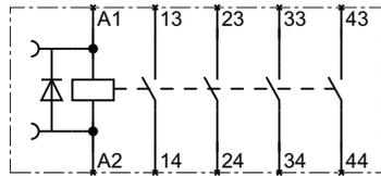
Contactor relay, with integrated diode, 4 NO contacts
