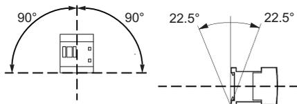
Figure 7-2 Mounting positions 3RT1.5, 3RT1.6 and 3RT1.7
