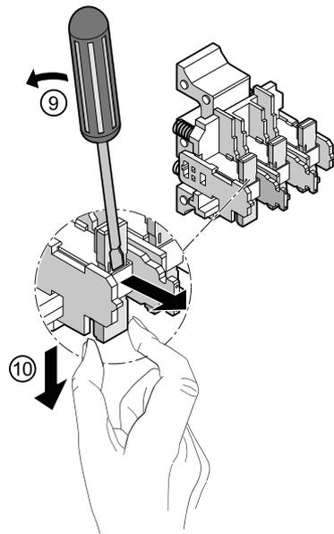
⑨/⑩ Use a screwdriver to lever the fixed contacts from the contact piece carrier.
