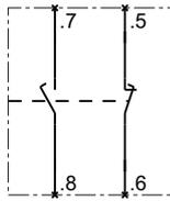
Auxiliary switch, 1 x make-before-break, 1 NO contact, 1 NC contact
