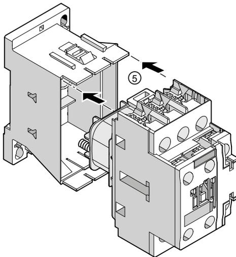
⑤ Reattach the front part of the contactor onto the rear half until the retaining clips engage.
