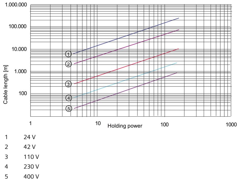
Figure 6-30 Graphical representation, switch-off
