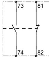
Auxiliary switch, for mounting on the front, 2-pole, 1 NO contact, 1 NC contact
