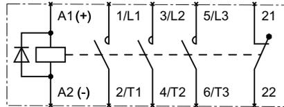
S00 contactor, with internal diode, 1 NC contact
