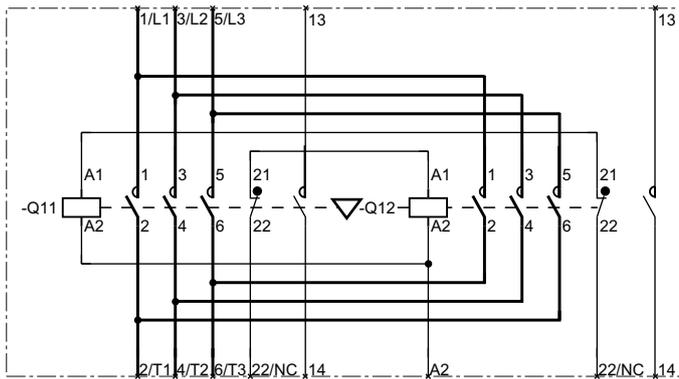
Figure 11-3 Reversing contactor assemblies S0, S2 and S3
