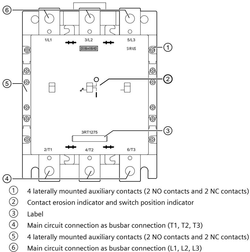
Figure 4-11 3RT1275-6LA06 vacuum contactor, size S12, overview
