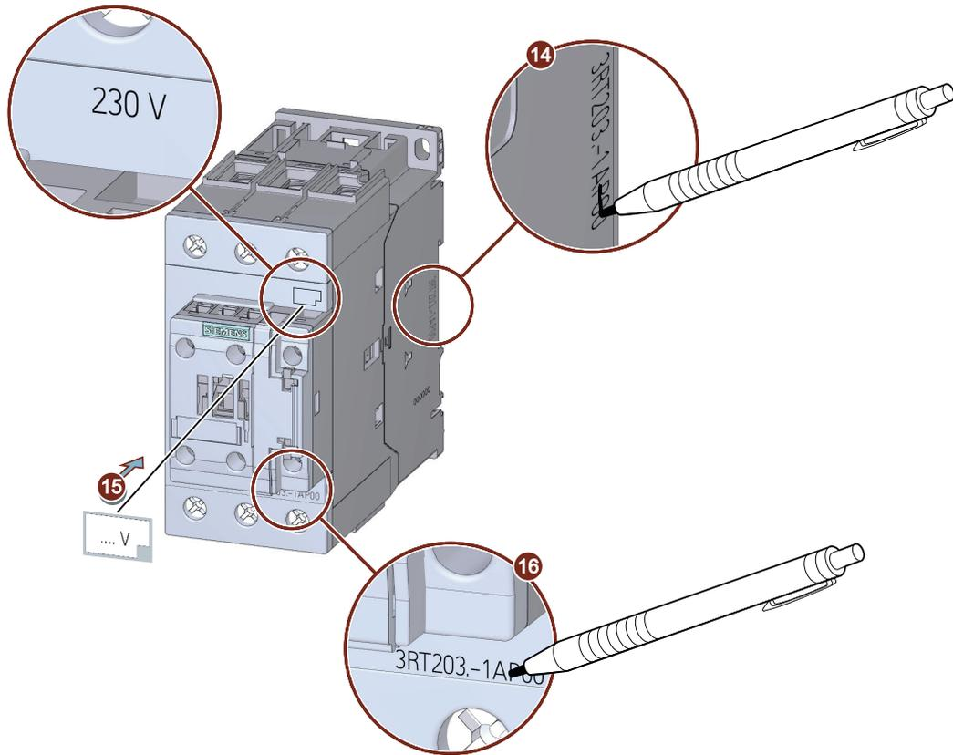
⑭/⑮/⑯ To label the coil voltage of the newly inserted operating mechanism, cover the control supply voltage specification with the labels supplied. Thoroughly cross out the article number.
