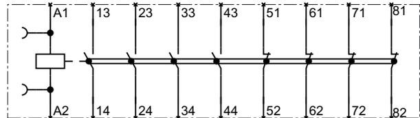
Contactor relay, without RC circuit, 4 NO contacts,
