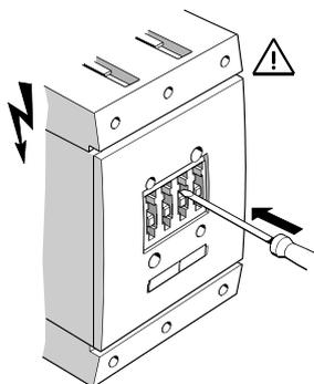
With 3RT105 / 3RT106 / 3RT107 / 3RT145 / 3RT146 / 3RT147 air-break contactors, the lateral auxiliary contacts can be operated for test purposes by pressing the auxiliary switch receptacle / switch position indicator on the front. By doing this the main contacts would also touch, without resulting in contact resilience.
