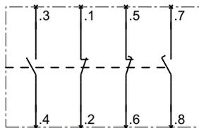
Auxiliary switch, for mounting on the front, 4-pole, 1 x make-before-break, 2 NO contacts, 2 NC contacts
