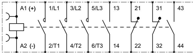
S0 / S2 / S3 contactor, without RC circuit, 2 NO contacts, 2 NC contacts
