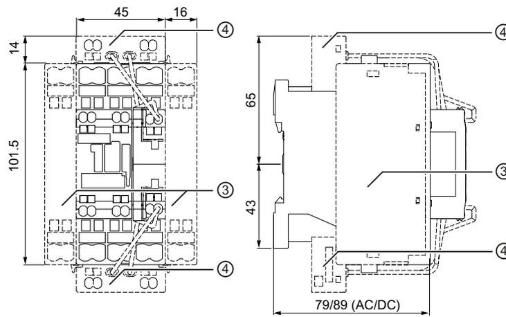
3 4-pole contactor for switching slightly inductive or non-inductive loads 3RT232.
