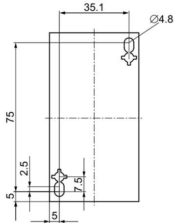
Figure C-24 Drilling plan for 3RT202.-4 contactors (size S0)
