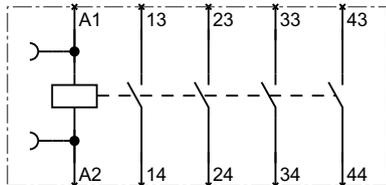
Contactor relay, without RC circuit,
