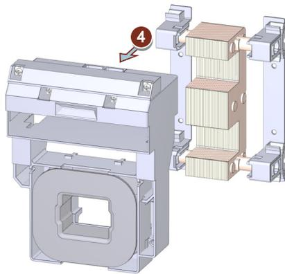
④ Remove the solenoid coil.
