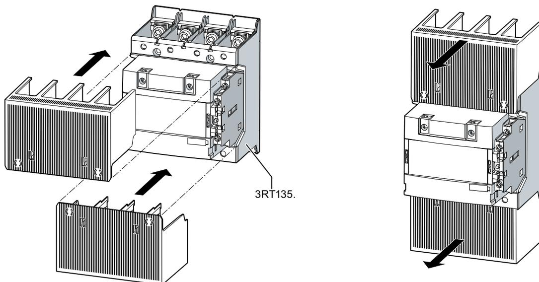
9.39 Terminal cover for 3RT135, 3RT136 and 3RT137 contactors (sizes S6 to S12)
