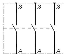
Auxiliary switch, for mounting on the front, 4-pole, 3 NO contacts
