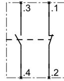
Auxiliary switch, for mounting on the front, 2-pole, 1 NO contact, 1 NC contact
