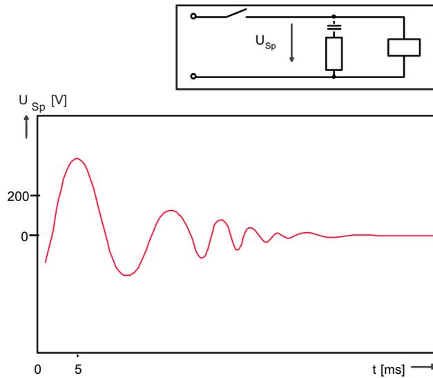
Figure 9-10 RC circuit with RC element (AC/DC operation)
