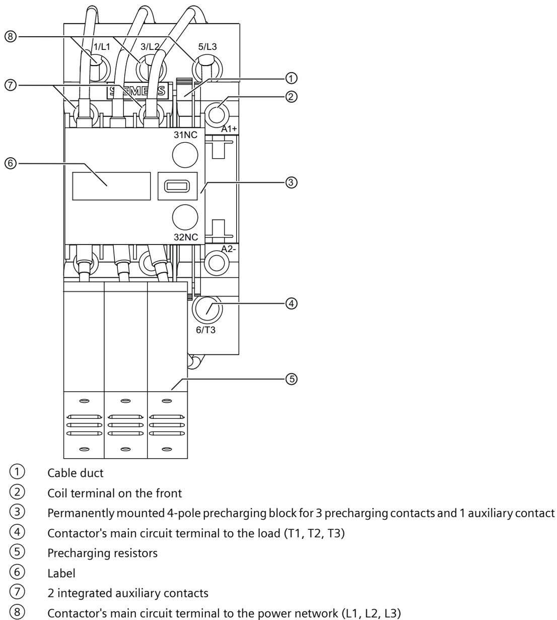
Figure 4-22 3RT2625-.....-..... capacitor contactor, size S0, overview
