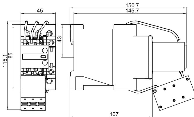
Figure C-39 3RT2625-1B... capacitor contactors (size S0)
