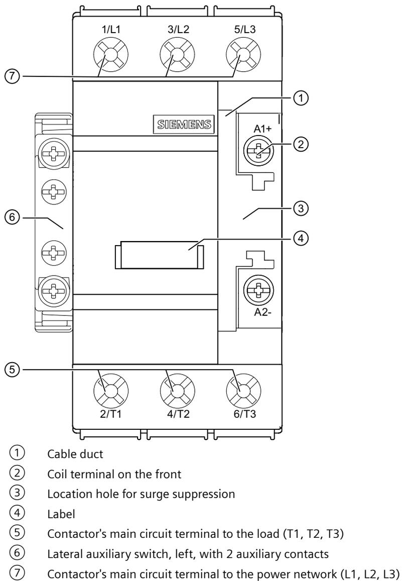
Figure 4-24 3RT263-.....-..... capacitor contactor, size S2, overview
