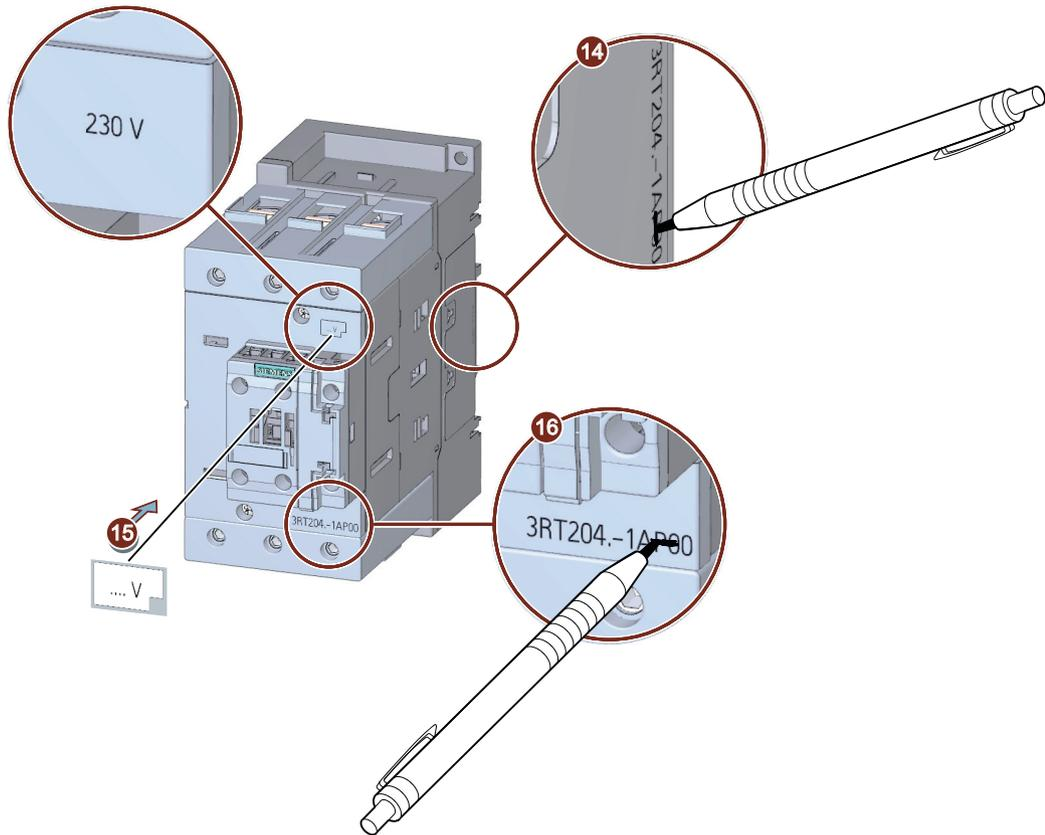
⑭/⑮/⑯ To label the coil voltage of the newly inserted operating mechanism, cover the control supply voltage specification with the labels supplied. Thoroughly cross out the article number.
