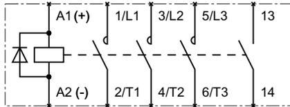
S00 contactor, with internal diode, 1 NO contact
