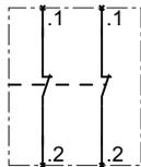
Auxiliary switch, for mounting on the front, 2-pole, 2 NC contacts
