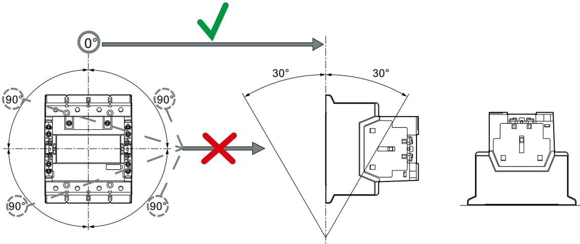
Figure 7-3 Mounting positions 3RT135, 3RT136 and 3RT137
