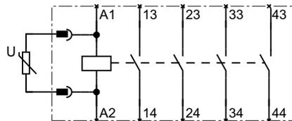
Contactor relay, with connected varistor, 4 NO contacts
