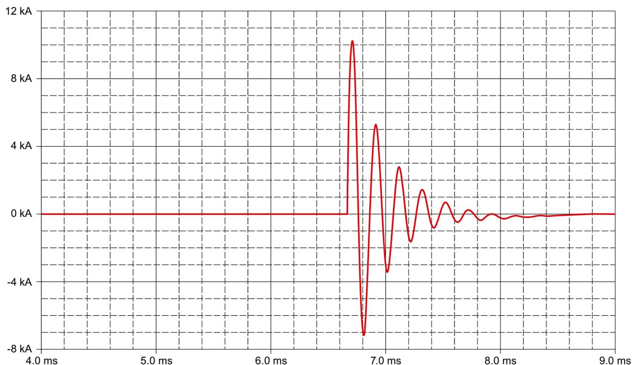
Figure 6-15 1. Energizing with contactor (without precharging)
