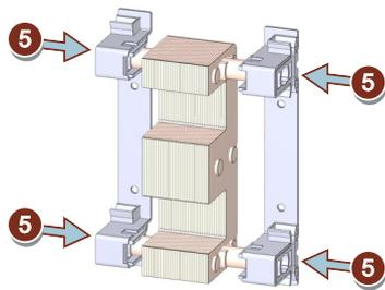
⑤ Slide both supports for the iron core together.
