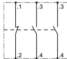
Auxiliary switch, for mounting on the front, 4-pole, 2 NO contacts, 1 NC contact
