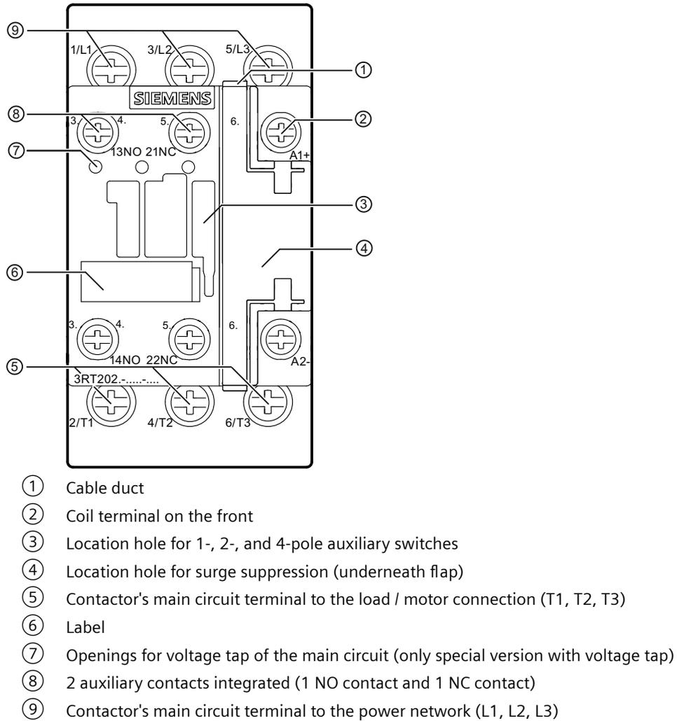
Figure 4-2 3RT202-.....-..... power contactor, size S0, overview
