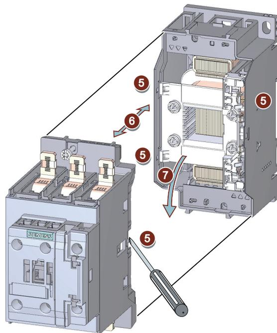
⑤/⑥/⑦ Push the two halves of the contactor apart. Note the lateral latching here. Take the solenoid coil out of the rear half of the contactor.
