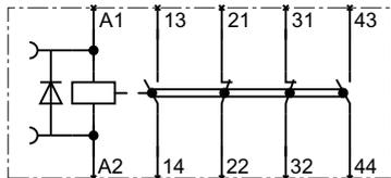
Contactor relay, with integrated diode, 2 NO
