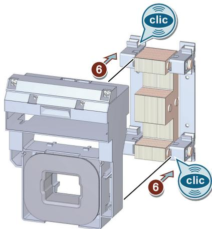
⑥ Slide the new solenoid coil onto the iron core.
