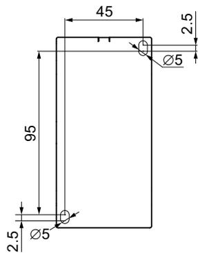
Figure C-30 Drilling plan for 3RT2.3. contactors (size S2)
