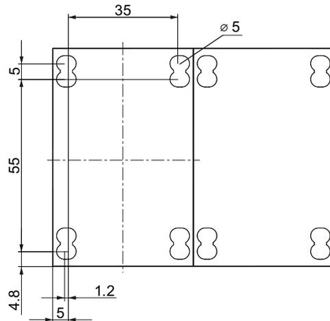
Figure C-50 Drilling diagram of the 3RA231.-8X.3.-2 reversing contactor assemblies (size S00, spring-loaded connection system)
