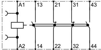
Contactor relay, without RC circuit,
