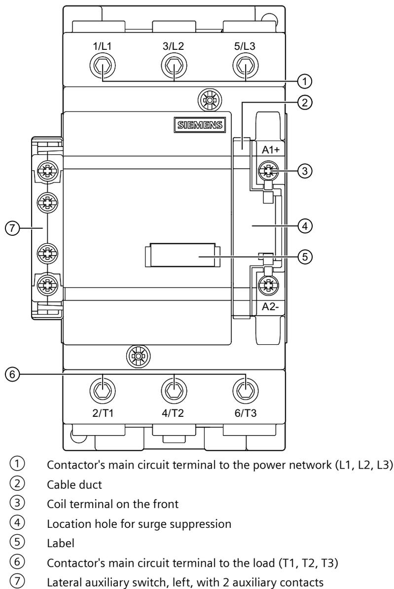
Figure 4-25 3RT264.-.....-..... capacitor contactor, size S3, overview
