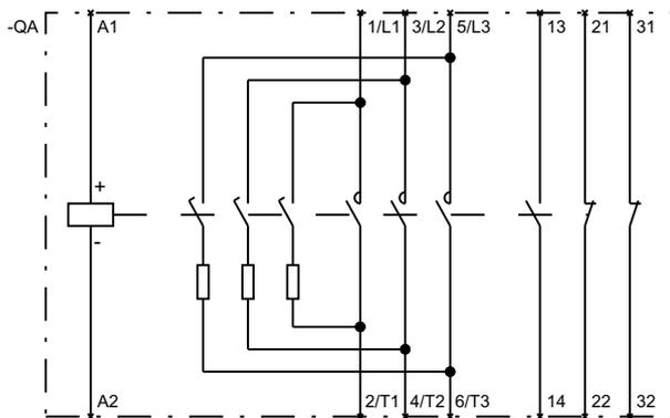
11.3 Capacitor contactors (S00 / S0 / S2 / S3)
