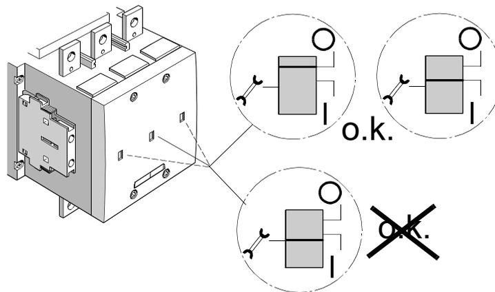
Figure 7-6 Contact erosion indicator and switch position indicator
