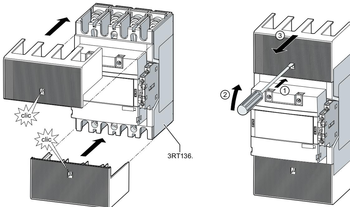
Mounting / disassembling the 3RT1976-4EB10 terminal cover
