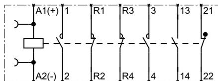
Pole-changing contactor, S0, S2 and S3, 4 main current paths, 2 NO contacts, 2 NC contacts, plus 1 NO contact, 1 NC contact
