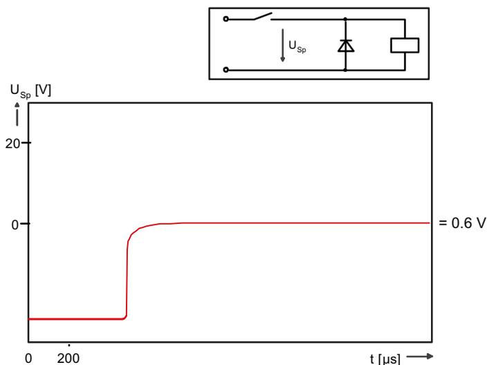
Figure 9-11 RC circuit with diode (DC operation)
