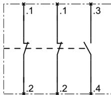
Auxiliary switch, for mounting on the front, 4-pole, 1 NO contact, 2 NC contacts
