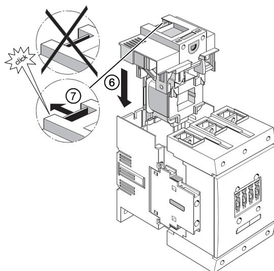
⑥ / ⑦ When re-installing, ensure that the interlock clearly engages again:
