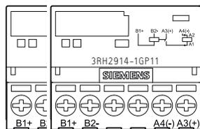
Figure 9-18 Terminals on the 3RH2914-.GP11 . coupling link
