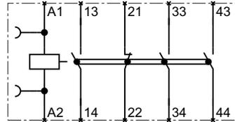
Contactor relay, without RC circuit, 3 NO contacts,
