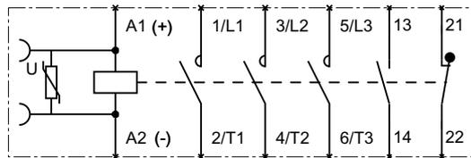
S0 / S2 / S3 contactor, with electronic operating mechanism, 1 NO contact, 1 NC contact
