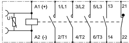
S0 / S2 / S3 contactor, with internal varistor, 1 NO contact, 1 NC contact
