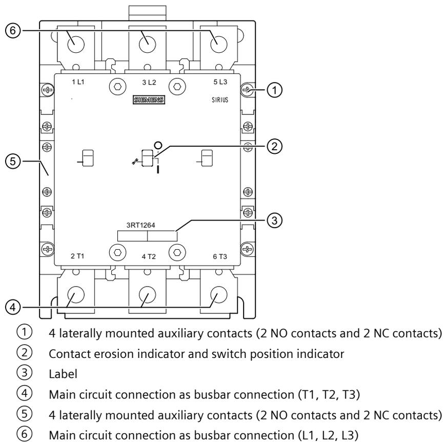
Figure 4-10 3RT1264-6LA06 vacuum contactor, size S10, overview
