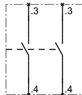
Auxiliary switch, for mounting on the front, 4-pole, 2 NO contacts
