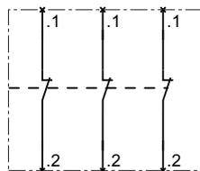
Auxiliary switch, for mounting on the front, 4-pole, 3 NC contacts
