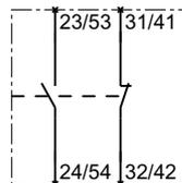
Auxiliary switch, lateral, 1 NO contact, 1 NC contact
