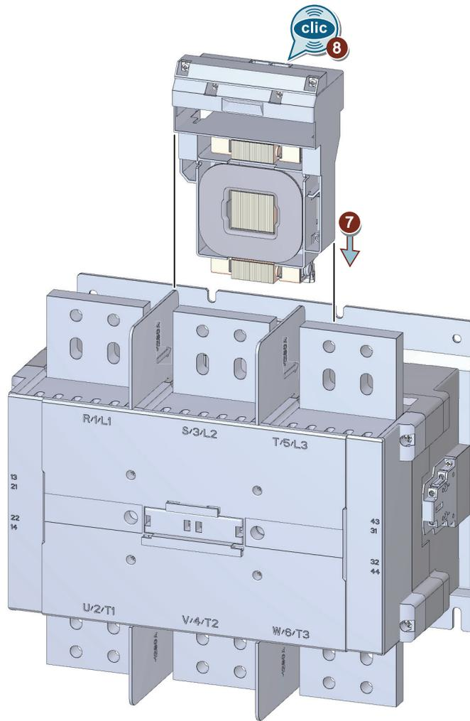
⑦ / ⑧ Make sure that the solenoid coil clearly engages on reinsertion.
