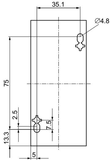
Figure C-23 Drilling plan for 3RT202.-2 contactors (size S0)
