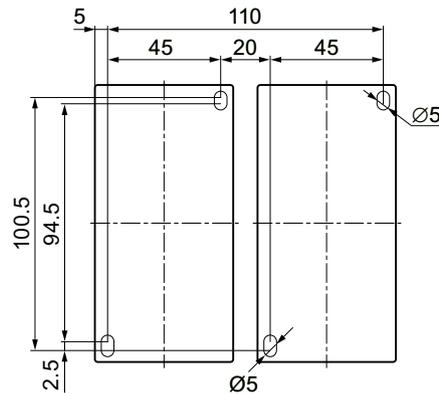
Figure C-58 Drilling diagram for 3RA233.-8XB30-1 reversing contactor assemblies
