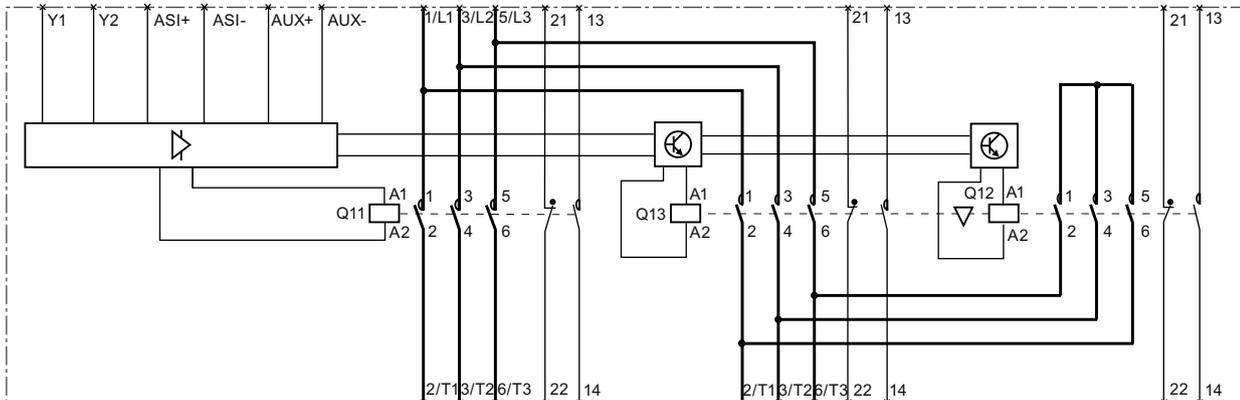
Figure 11-7 S0, S2 and S3 contactor assemblies for star-delta (wye-delta) start, with mounted function modules for AS-Interface
