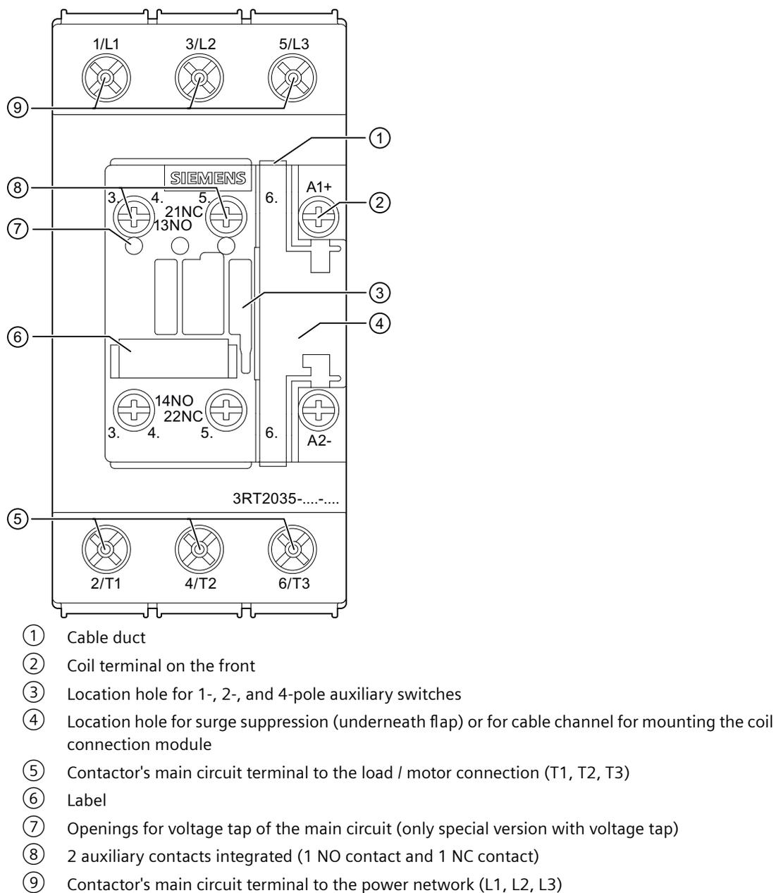
Figure 4-3 3RT203-..... power contactor, size S2, overview
