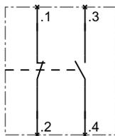
Auxiliary switch, for mounting on the front, 4-pole, 1 NO contact, 1 NC contact
