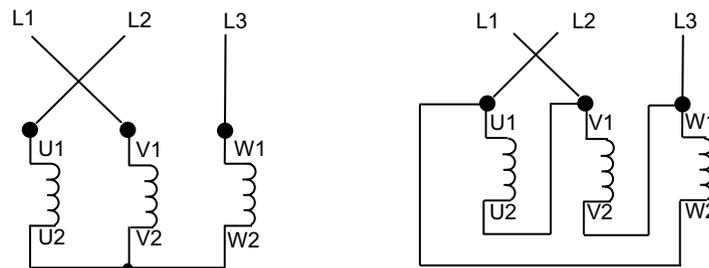
Figure 6-25 Correct connection of motor phases for counterclockwise motor rotation
