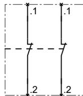
Auxiliary switch, for mounting on the front, 4-pole, 2 NC contacts
