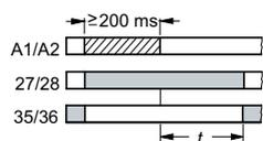
OFF-delay without auxiliary voltage
