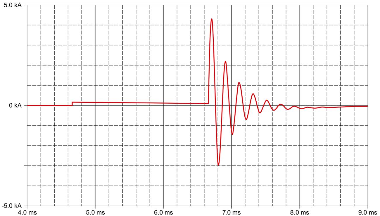
Figure 6-16 2. Energizing with a 3RT2636 capacitor contactor (with precharging)
