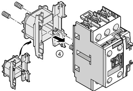
④ Insert the new solenoid coil. In doing so, make sure that the springs between the solenoid coil and the front half of the contactor are properly located on the support.
