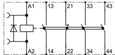
Contactor relay, with integrated diode, 3 NO
