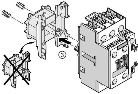
③ Take the solenoid coil out of the front half of the contactor.
