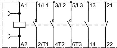
S0 / S2 / S3 contactor, without RC circuit, 1 NO contact, 1 NC contact
