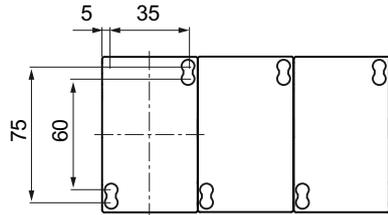
Figure C-64 Drilling diagram for 3RA242.-8X.3.-1 contactor assemblies for star-delta (wye-delta) start (size S0, screw-type connection system)
