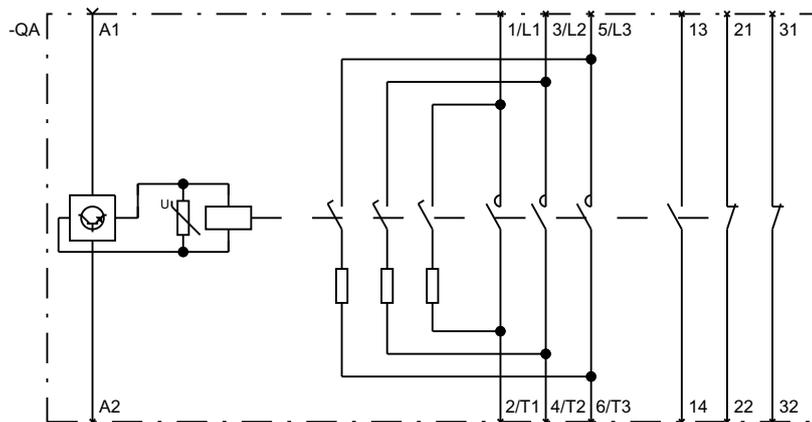
Capacitor contactors (sizes S2 and S3)
