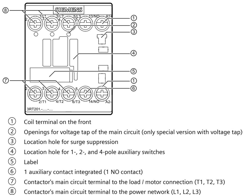
Figure 4-1 3RT201.-..... power contactor, size S00, overview
