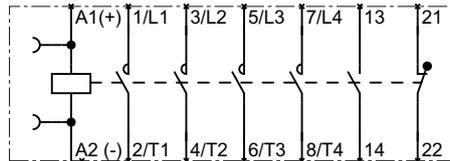
S0, S2 and S3 contactor, 4 main current paths for switching slightly inductive loads or non-inductive loads, 4 NO contacts plus 1 NO contact, 1 NC contact
