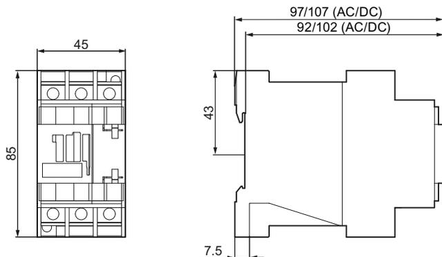
Figure C-20 3RT2.2.-4 contactors (ring cable lug connection system)
