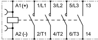
S00 contactor, without RC circuit, 1 NO contact
