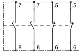
Auxiliary switch, for mounting on the front, 4-pole, 2 x make-before-break, 2 NO contacts, 2 NC contacts
