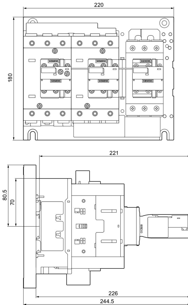
**C.17.4.2 Drilling diagram for 3RA244.-8X.32-1 contactor assemblies for star-delta (wye-delta) start (size S3)**
