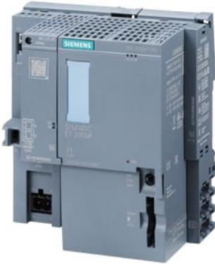
SIMATIC DP, CPU 1510SP-1 PN for ET 200SP, central processing unit with work memory 200 KB for program and 1 MB for data, 1st interface: PROFINET IRT with 3-port switch, 6 ns bit performance, SIMATIC Memory Card required, BusAdapter required for port 1 and 2
