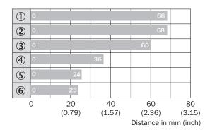
$\begin{tabular}{ll} \hline & Max. sensing range $S_n$, flush or non-flush installation, \\ & non-magnetizable material \\ \hline \end{tabular}$
