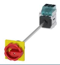
3LD3 switch disconnector, Iu 32 A main switch 3-pole rated operational power for AC-23 A at 400 V 11.5 kW floor mounting basic switch with door coupling centerhole mounting 22.5 mm rotary operating mechanism red/yellow 66 x 66 mm with auxiliary switches 1 NO + 1 NC
