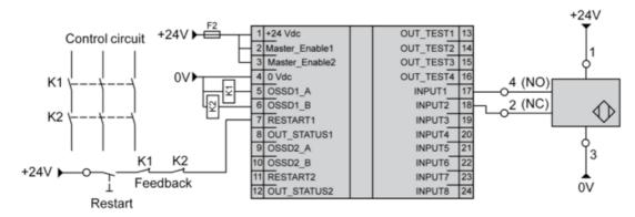
SFF : (Safe Failure Fraction): 92,68 % DC : (Diagnosis Coverage): 75,8 %
