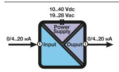
Z109S-DI is a device that allows to isolate and convert a 0/4 - 20 mA signals. The device can power also all 2-wire sensors providing a stabilized voltage of 20 V and a max current of 20 mA with short-circuit protection. A 3-way galvanic isolation of 3.500 Vac among Power supply // input // output circuits assures the integrity of your data.
