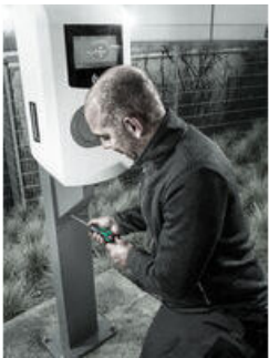
Torque screwdriver with quick torque adjustment
