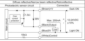
\*\*Before using this unit, select Light ON/Dark ON with control cable. (Light ON: Connect control cable with 0V/Dark ON: Connect control cable with +V) \*Control cable is only for Diffuse reflective/Narrow beam reflective/Retroreflective type
