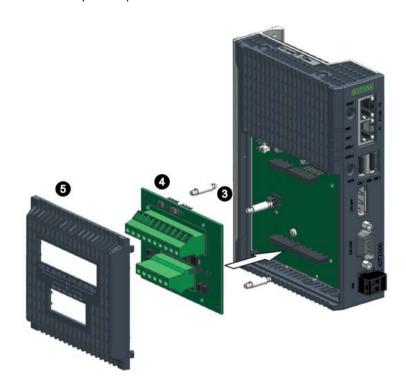
5. Install the Input/Output module cover to the IOT2050.
