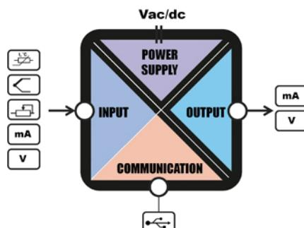
Z109REG-BP is a converter with universal input in voltage (mV), current (mA), thermocouples (TC), thermoresistance (RTD), potentiometer, rheostat, NTC.
