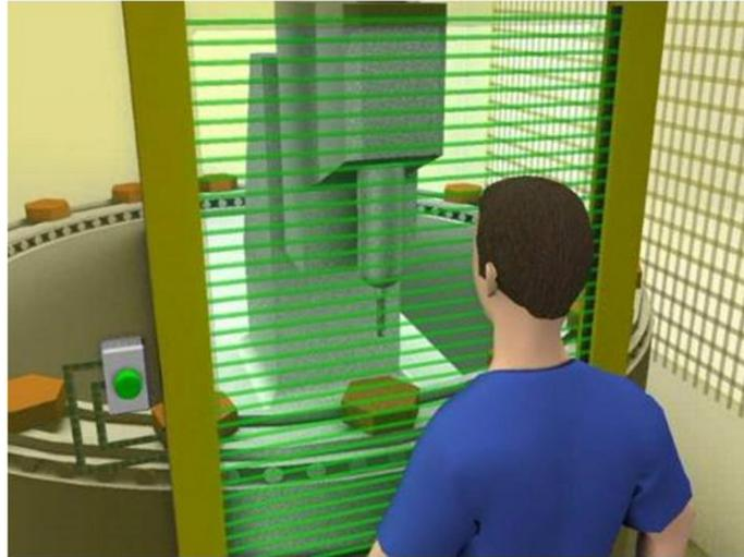
Fig 5 - Operating point protection on drilling machines
