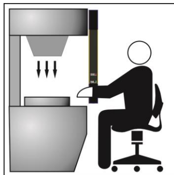
Fig. 7 - Correct light curtain positioning
