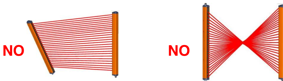
Fig. 17 - Wrong light curtain TX-RX orientations
