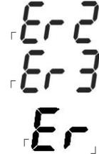
'Er2' is displayed when the thermometer is exposed to rapid changes in the ambient temperature. 'Er3' is displayed when the ambient temperature exceeds 0°C(32°F) or +50°C (122°F).
