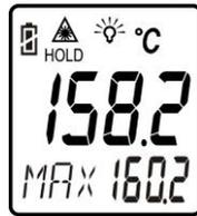
1. Simply aim the thermometer at the measure target with Lens (○,9) and press Meas. key (○,7) to display the surface temperature.
