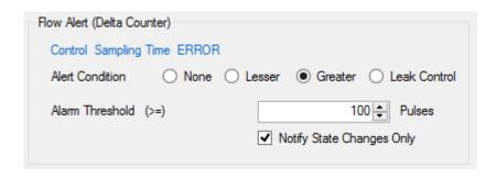
**Leak Control** the alert is activated if in the report period time the minimum of the delta sample is lesser than threshold. The Leak control can be used for pipes leak control: there must be a sample period where the consumption must be near to 0:
