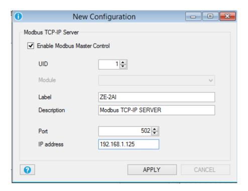
Select the Modbus TCP-IP Server *UID* (unit id or node id), then enter a Modbus Server label.
