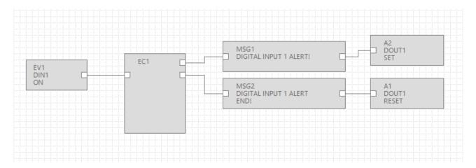
Configure the EC1 block for routing the alert condition in state S1 and the alert end condition in state S2:
