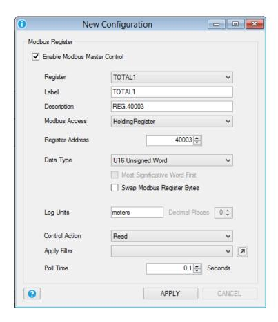
Select the register from the slave module database (all the others items will be automatically adjusted).
