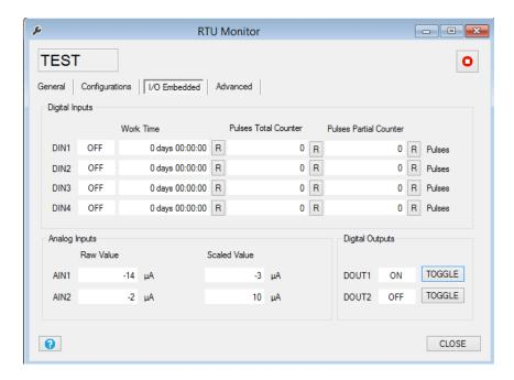
**Digital Inputs** show the Digital input state ON/OFF, the work time input. Also are presents the Total and Partial counters (raw values not scaled).
