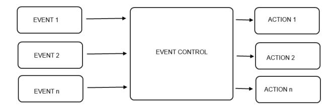
One or more *events* must be connected to an *event control*, this block performs the logic and select the right *action* output.
