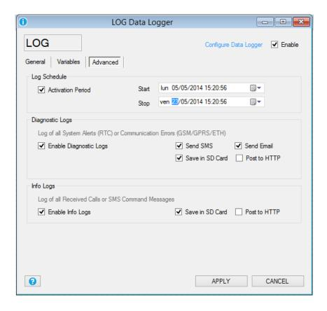
**Activation Period:** If checked enable the start date and a stop date of the datalogger, if disabled the datalogger is always on.
