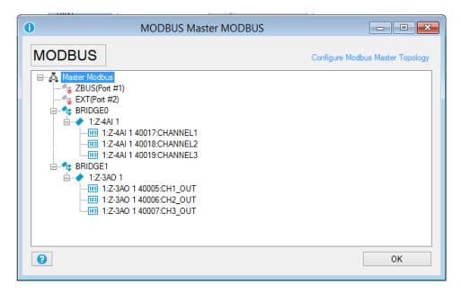
We use the analog copy block for read (using Modbus TCP-IP) from the Z-4AI channels an write to the Z-3AO channels:
