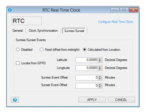
With a sophisticated algorithm, the RTU can calculate the Sunrise and Sunset events from the GPS coordinates and from the Date/Hour. So it's possible to use the events for turn on/off a lamp, stop the datalogger etc..
