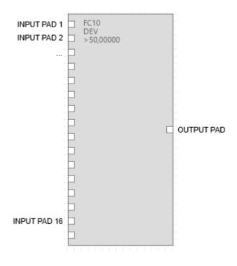
This block function calculate the absolute difference between an input and the average of all the inputs, than compare all this values with a threshold, if at least one of these compares is true the output is true too.
