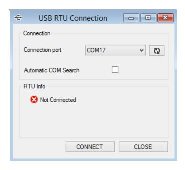
**Connection port** is the serial port connected to the PC, select the right Z-GPRS2/Z-logger virtual com port, note that you must first connect the Z-GPRS2/Z-Logger and then after.
