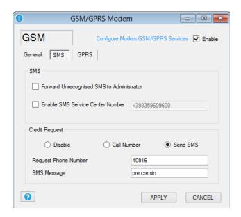
This window will configure the modem SMS functions:
