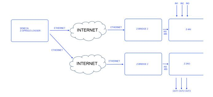
The modbus configuration use a Z-Bridge2 connected with a Z-4AI, then another Z-Bridge2 with a Z-3AO:
