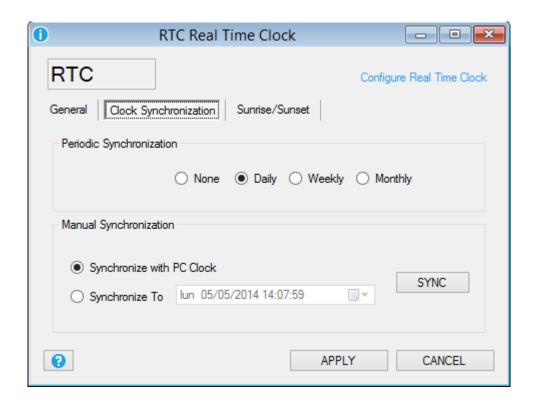
**Periodic Synchronization:** Select the synchronization time for the Ethernet Network Time Protocol or GPRS automatic synchronization
