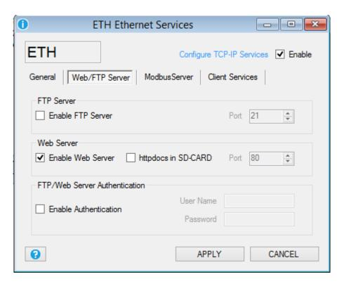
**FTP Server:** If checked enable the internal FTP server, the FTP server file system is the microSD card so you can acquire the log files directly from the FTP server. For use an FTP client remember to force the "only one connection" option, for example in filezilla ftp client:
