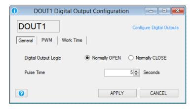
Digital Output Logic: Select the Normally Open or Normally Close output logic.
