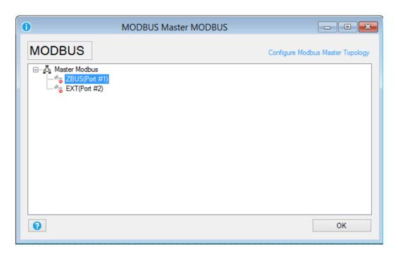
Configure the external IO connected to the Modbus RTU Port #1 and Port#2, also the Modbus TCP-IP client can be configured here. Up to 100 Modbus RTU/TCP-IP TAGs can be configured.
