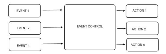
The EC inputs accept boolean events, each event control output must be connected to an action.
