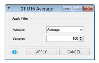
The average filter is used for obtaining a moving average on the selected numbers of samples.
