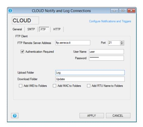
FTP Remote server Address: Enter the remote FTP server ip address or name.
