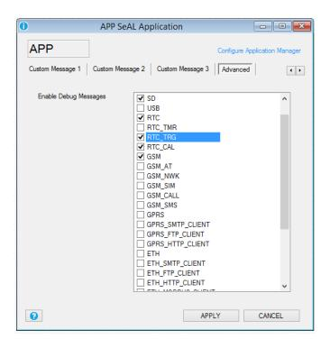
Using the debug port, you can view and save to a file a log of operations performed by the RTU. To connect to the debug port you must use the USB adapter "Easy USB", buy-it directly on the site Seneca (www.seneca.it) or contact Seneca for more info:
