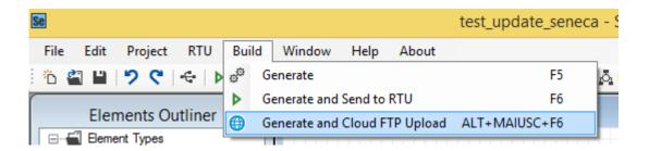
This function will copy to the download ftp folder the "RTUNAME\_fwupdt.tag" and the "RTUNAME \_setup.tag" files, where RTUNAME is the RTU name from the Cloud-General Form, for example:
