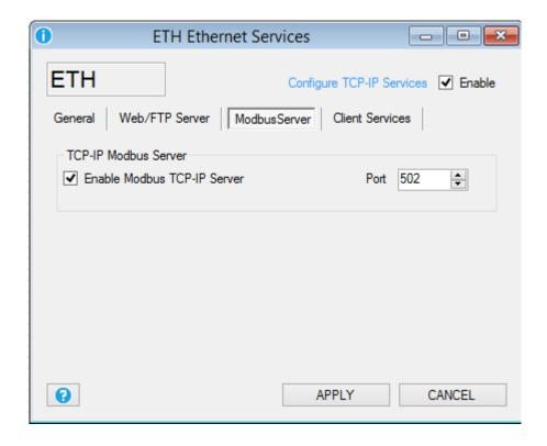
**Enable Modbus TCP-IP Server:** if checked enable the Modbus TCP-IP server, so it's possible to read the real time values of variables directly from a SCADA or an external display, PC etc...
