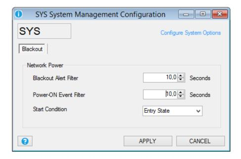
**Blackout Alert Filter:** Select for how much seconds the main power must continuously be down before the RTU send an alert of blackout.
