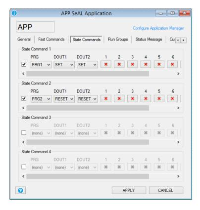
Select the PRG1 or PRG2 command (defined in the General section) or/and the Digital Out function.
