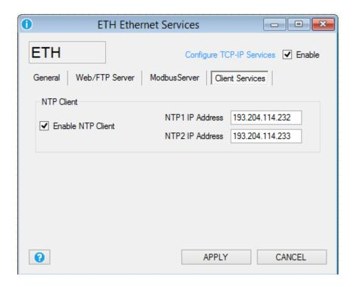
**Enable NTP Client:** If checked enable the Network Time Protocol used for synchronize the RTU Date/Time.
