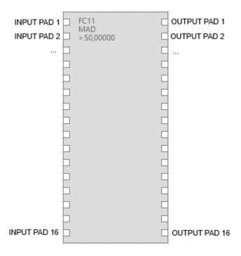
This block function calculate the absolute difference between each input and the average of all the inputs, than compare each of these values with a threshold. The compare output is emit to each output pad (input 1 compare to output 1, input 2 compare to output 2 and so on).
