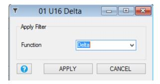
The delta filter is used for obtaining the difference between two consecutive Modbus Value read.
