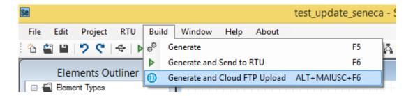
This function will copy to the download ftp folder the "RTUNAME\_fwupdt.tag" and the "RTUNAME\_setup.tag" files.
