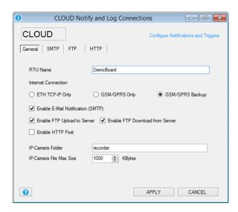
RTU Name: Enter the RTU Name, this name is also the prefix of the .csv log file name.
