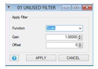
The scale filter is used for apply a scale factor to the Modbus value, the filter result is obtained by the relation:
