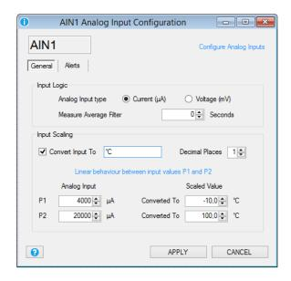
Analog Input Type: Select the analog input type from current (from 0 to 20 mA) or voltage (from 0 to 30 V).
