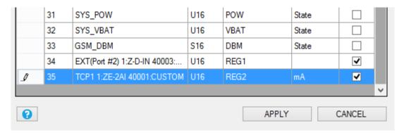
Note that if you have applied a filter to the modbus value only the filter output value will be logged.
