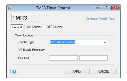
**Counter Type:** select from ON timeout counter (use only the ON action and the ON timeout), OFF timeout counter (use only the OFF action and the OFF timeout), ON/OFF use ON and OFF timeout counters, ON WorkTime (use only the OFF action and the OFF timeout), OFF WorkTime (use only the OFF action and the OFF timeout), ), ON/OFF Worktime use ON and OFF timeout counters.
