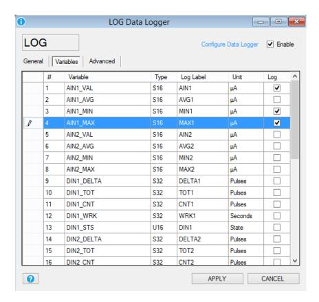
Select the TAGs that you want to log by flagging the Log column, Double click on the "Log label" column for changing the variable label. The Modbus Tags are at the end of the window:
