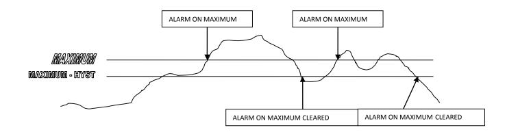
If the threshold is Minimum or Low the alarm is activated when the analog input is < threshold but the alarm rearm is obtained when at the analog input is > (Threshold+Hysteresis).
