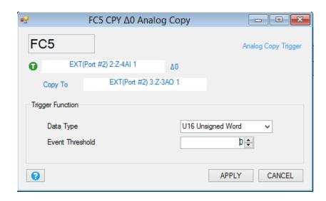
*Data Type:* Select the input and output data type from Integer Signed 16 Bits , Integer Signed 32 Bits or Floating point 32 Bits.
