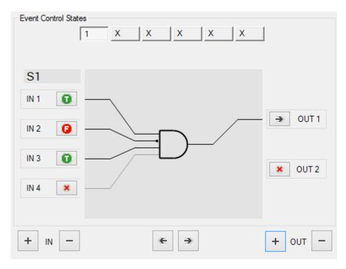
In this example if IN1=True, IN2=False and IN3=True, the Action connected to the OUT1 is executed.
