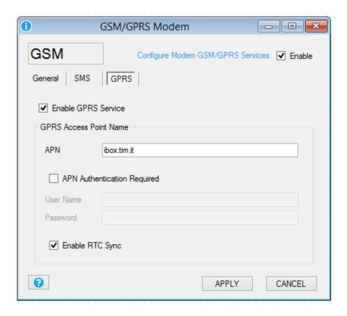
**Enable GPRS Service:** if checked activate the GPRS internet connection.
