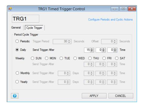
Period Cycle Trigger: select how often execute the cycle trigger action.
