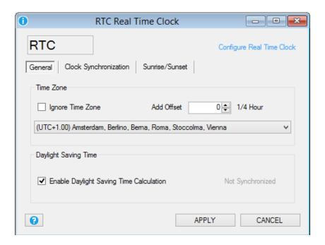
**TIME ZONE:** configure the RTU installation timezone, it's possible to ignore timezone for set a custom Date/Hour with SEAL software or set the right timezone. If you are using the Network Time Protocol (NTP) from Ethernet or the GPRS for synchronize data/hour you must configure the right Timezone because the server hour is UTC (Universal Time Coordinating). The UTC and GMT (Greenwich Medium Time) can be defined as equal.
