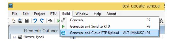
This function will copy to the download ftp folder the "RTUNAME\_fwupdt.tag" and the "RTUNAME \_setup.tag" files, where RTUNAME is the RTU name from the Cloud-General Form, for example if RTUNAME = ZGPRS1588:
