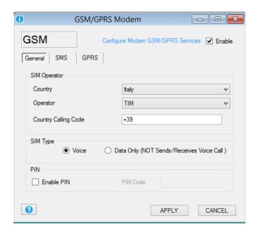
This window will configure the GSM/GPRS modem (only for model Z-GPRS2).
