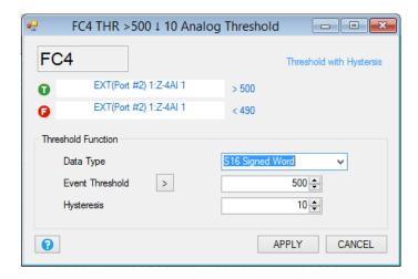
*Data Type:* select the input data type from Integer Signed 16 Bits , Integer Signed 32 Bits or Floating point 32 Bits.
