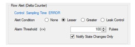
*Greater* the alert is activated if the delta is greater than threshold:
