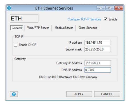
**Enable DHCP:** If checked enable the Dynamic Host Configuration Protocol, the IP address, and the Subnet mask are obtained automatically from the DHCP server (often the router/gateway).
