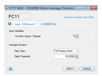
*Function Inputs/Outputs:* Select the input/output pad numbers (from 2 to 16). Note that you can't leave unconnected an input pad.
