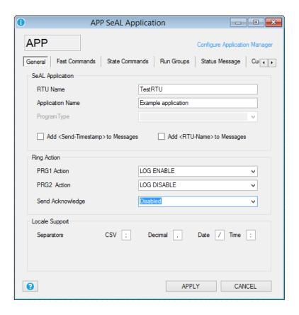
RTU Name: Insert the RTU name
