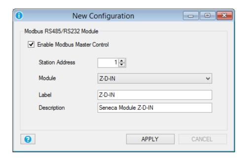
Select the slave station address and the Module name from the Seneca module database. If your slave is not in the database select "*custom*" for customize a slave module.
