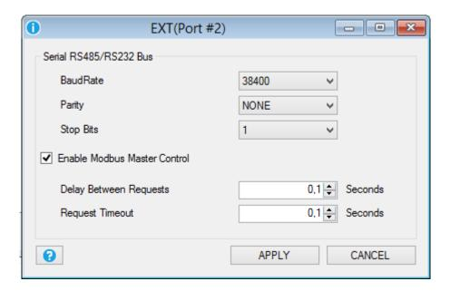
Select the Buad Rate, the parity and the stop bits agree to the connected modbus RTU slaves devices.
