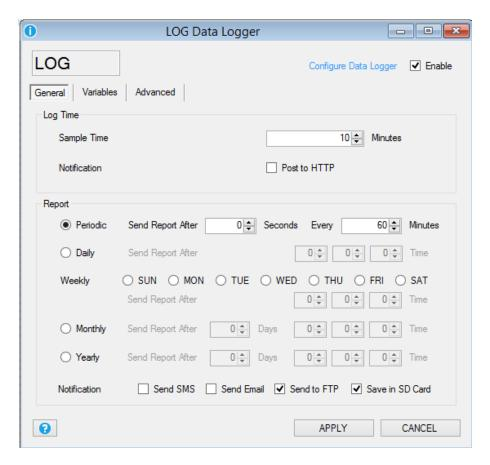
The Data Logger configuration can setup which TAG must be logged, how often acquire and how often send data to the cloud.
