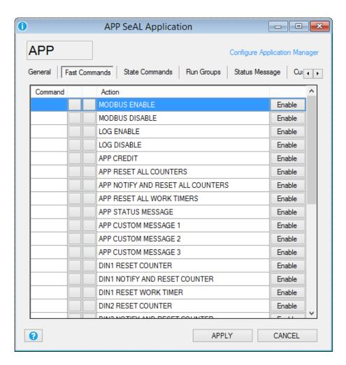
Select the "Enable" button for selecting the Command to enable from the commands database:
