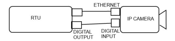
*IP Camera Folder:* Configure the RTU FTP Server where the IP camera will put videos and/or snapshots. When a new file is written in this folder the RTU will send the data from the Log notification channel configured (Ethernet or GPRS) to the profiles that includes the logs group. When a file is correctly sent the RTU will delete it from the local ftp.
