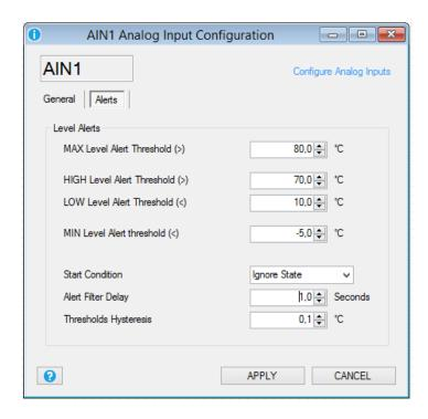
Maximum Level Alert Threshold: The alert is activated if the analog input is > Max Level configured.
