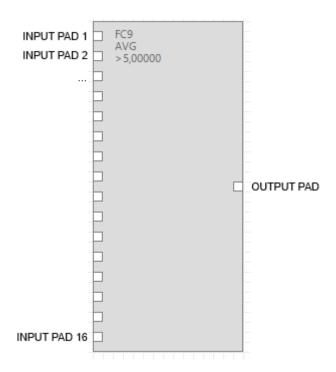
This block function calculate an average of all the inputs, than compare this average with a threshold.
