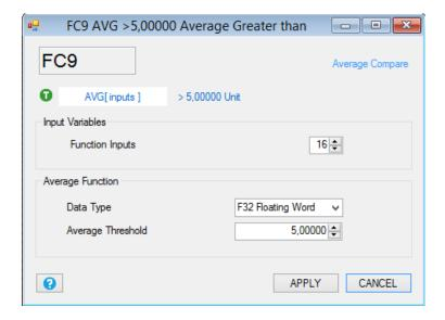
**Function Inputs:** Select the input pad numbers (from 2 to 16). Note that you can't leave unconnected an input pad.
