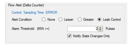
For example, considering a plumbing plant that supplies 2 utilities. Statistically, during one day (report time T = 24 hours) the admitted flow must be <0.1 m3/h (maximum admitted flow Q=0.1 m3/h) for at least one of the 10 minute t (sample time t= 10 minutes).
