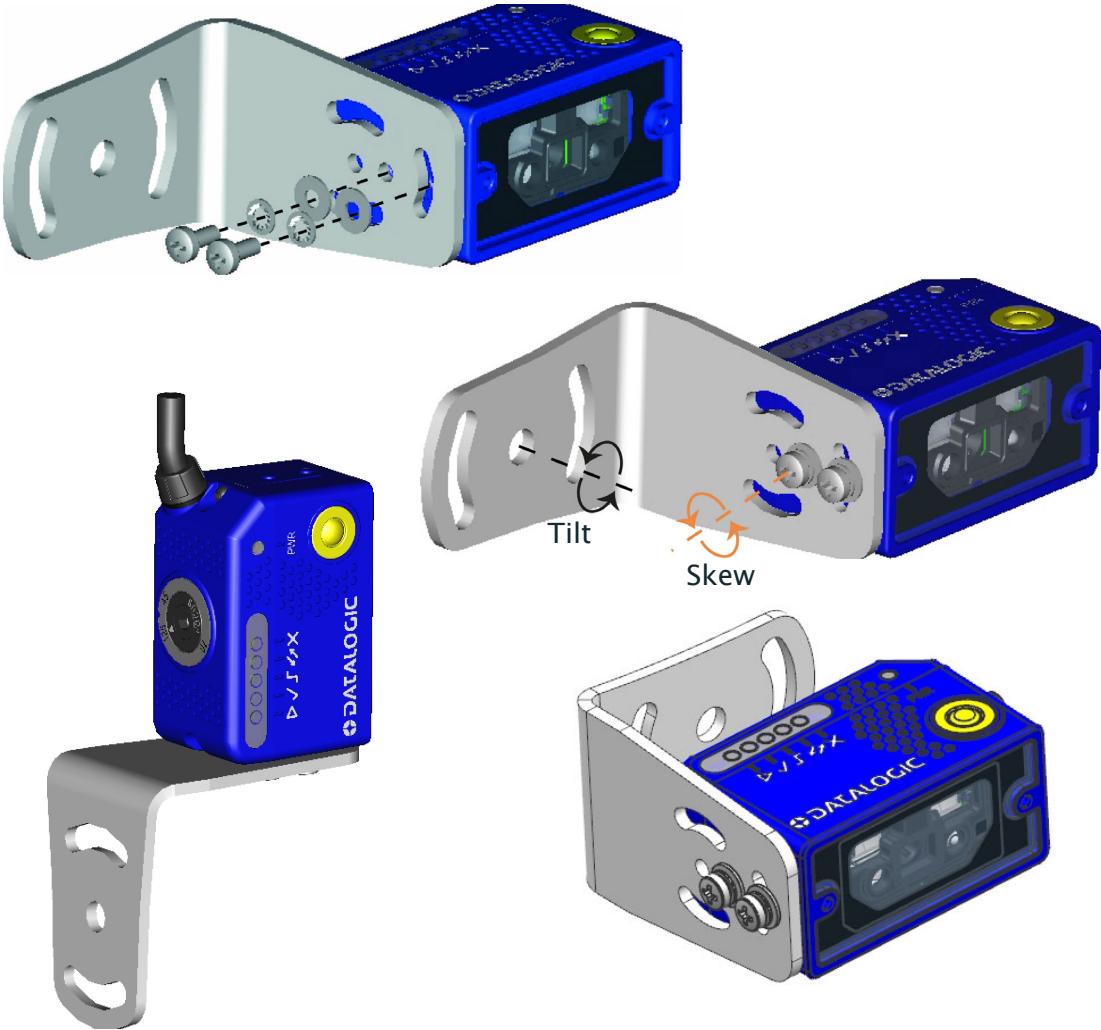
Figure 30 – Side Mounting Positions for USB Models
