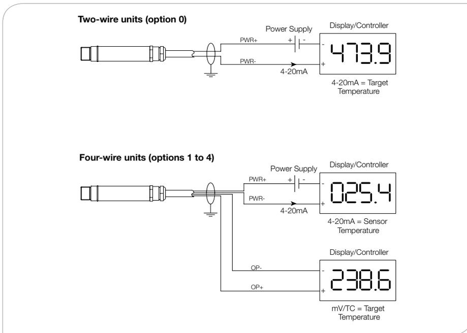
The PyroCouple Series is a range of high quality, low cost, compact sensors which measure the temperature of inaccessible or moving objects and materials. They measure temperatures from -20°C to 500°C, accurately and consistently, with an outstanding response time of 240 ms.
