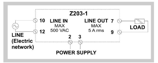
Connect to the screw terminals 10 and 12 the electric network. Connect to the screw terminals 7 and 9 the load to analyze.
