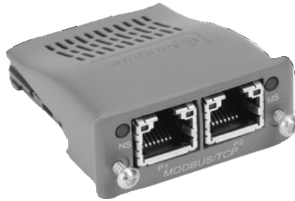
Figure 4.2.1 Modbus TCP Communication Module (AB6223)
