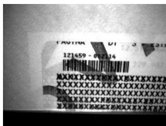
Figure 18 - Overprinted Barcode Readable by Matrix 120 also Through the Envelope Window Film
