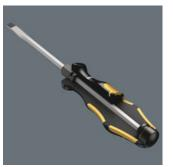
Wera makes its Kraftform handles from several materials with different properties. The core is made from a hardwearing plastic that holds the blade securely even when subjected to great forces. The yellow soft zones of the external mantle consist of a softer material with more friction resistance for high torque transfer. The black areas with a harder surface prevent the hand from sticking to the handle enabling you to adjust your grip more quickly.
