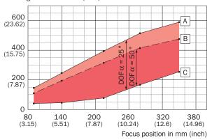
For devices with plastic reading window, the depth of field is reduced by approx. 10 %.
