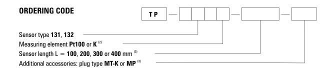
**Example for order**: TP-131Pt100-200-MP Pt100 resistance sensor of outer diameter  $\emptyset = 4 \text{ mm}/6 \text{ mm}$  length L = 200 mm
