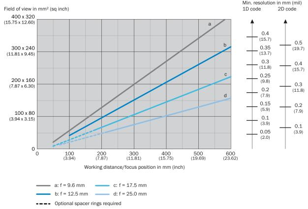
For S-mount and standard C-mount lenses, spacer rings are needed for working distances shorter than approximately 10 times the focal length. For compact C-mount lenses, spacer rings are not needed, but the built-in illumination cannot be used for distances shorter than 300 mm.
