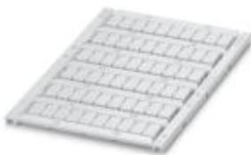
Marker for terminal blocks, Sheet, white, unlabeled, can be labeled with: TOPMARK NEO, TOPMARK LASER, BLUEMARK ID COLOR, BLUEMARK ID, BLUEMARK CLED, THERMOMARK PRIME, THERMOMARK CARD 2.0, THERMOMARK CARD, mounting type: snap into tall marker groove, for terminal block width: 6.2 mm, lettering field size: 5.6 x 10.5 mm, Number of individual labels: 60
