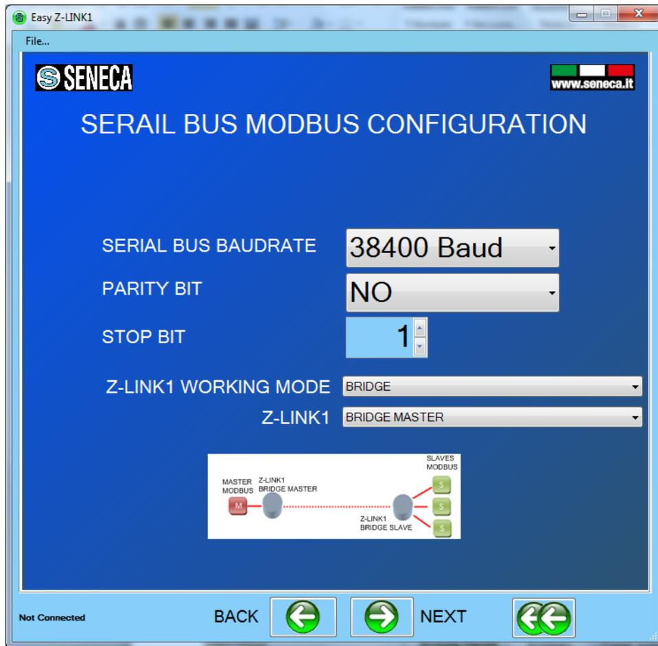
The Z-Link1 connected to the Master is called “Bridge Master”, the others Z-LINK1 (connected to the slaves) are called “Bridge Slave”.
