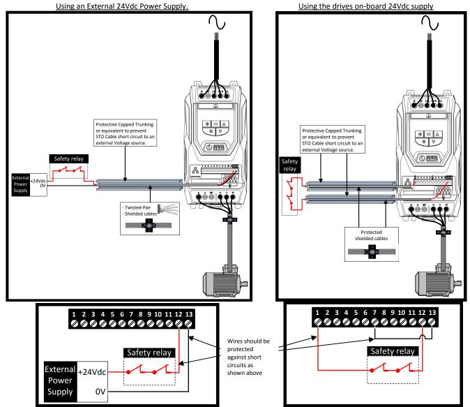
Note : The Maximum cable length from Voltage source to the drive terminals should not exceed 25 metres.
