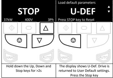
Note: Parameters cannot be defaulted whilst P2-39=1 (parameter set locked).
