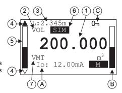
A, Calculated value of the output current. After the dimension, the mode of current output is indicated by inverse inscription:
