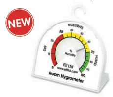
The general purpose hygrometer incorporates a 70 mm diameter dial with arrow indicator and colour-coded zones to display humidity levels e.g. dry, moderate and humid. The hygrometer indicates the level of humidity in 5 % divisions over the range of 0 to 100 %rh.
