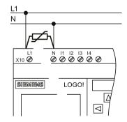
To suppress surge voltages, install varistors (MOV) with an operating voltage at least 20% above the rated voltage.
