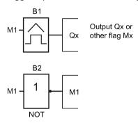
2. Configure the threshold trigger as shown below. LOGO! generates a pulse in each program cycle due to the inverted flag. The trigger interval is 2 seconds.
