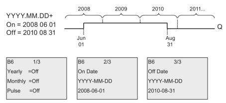
**Example 6:** Yearly mode off, Monthly mode off, Pulse selected, On Time = 2008-03-15, Off Time = \*\*\*\*-\*\*: on March 15, 2008 the timer output switches on for one cycle. Because the timer does not have a monthly action or yearly action, the timer output pulses only one time at the specified On Time.
