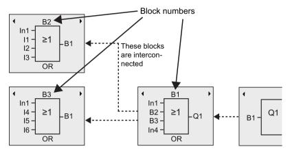
The figure above shows you three views of the LOGO! onboard display, which represent the circuit program. As you can see, LOGO! interconnects the blocks using their numbers. To scroll the circuit program, use the keys ◀ or ▶.
