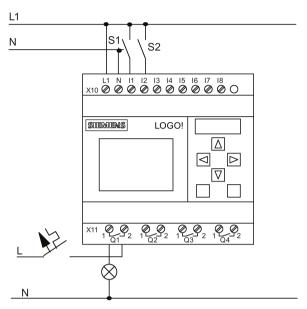
S1 switches input I1, while S2 switches input I2. The load connects to the relay Q1.
