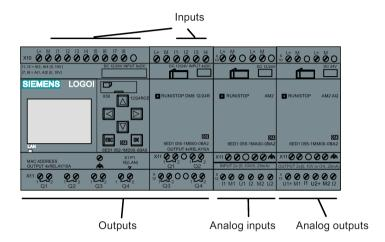
The illustration shows the conceptual usage of the inputs, not the actual physical markings on the module.
