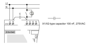
Take into account the quiescent current of any two-wire proximity switches that you use. The level of the quiescent current of some two-wire proximity switches is high enough to trigger a logical "1" signal at the LOGO! input. You should therefore compare the quiescent current of the proximity switches with the technical data of inputs (Page 322).
