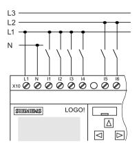
The inputs of these devices are in two groups, each consisting of four inputs. Different phases are only possible between blocks, but not within the blocks.
