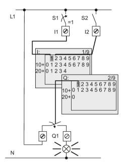
When switch S1 is closed, the status at input I1 is high.
