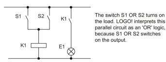
Translated into a LOGO! circuit program, you use an OR block to control relay K1 at output Q1.
