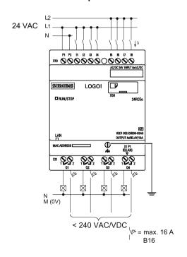
The inputs of these devices are not isolated and therefore require a common reference potential (chassis ground).
