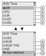
The current setting of automatic S/W Time conversion is indicated by a circle with a dot. The default setting is "④": disabled.
