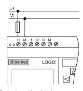
Protection with safety fuse if required (recommended) for: 12/24 RC...: 0.8 A 24: 2.0 A
