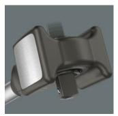
Changing the ratchet direction using a hardened push-through square drive ensures great resilience, since there is no susceptible switching mechanism that could be damaged by hammer blows. This is far more robust than a right/left switch.
