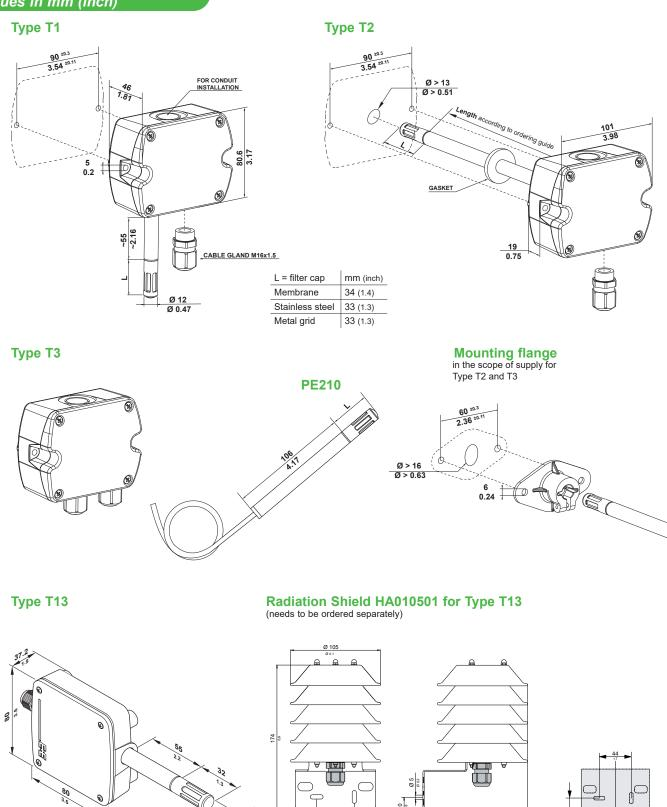
**EE210** with cable gland: Use a matching wrench to install the cable gland (in the scope of supply) onto the EE210 enclosure. **EE210** with conduit connection for the North American market: use a flat screwdriver to knock open the blind, carefully, in order to avoid damaging the electronics inside the enclosure. The conduit adapter is not included in the scope of supply. The M16x1.5 opening for the cable gland shall be tightly closed using the blind plug included in the scope of supply.
