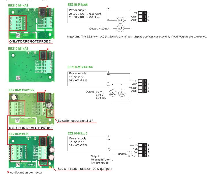
The PE210 (remote probe for EE210-M1T3x) shall be ordered and it is supplied as separate item. PE210 is to be connected to the EE210 by the user.
