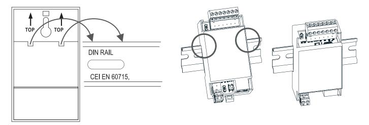
**Installation:** Position the device on the OMEGA rail resting the upper teeth from top to bottom.
