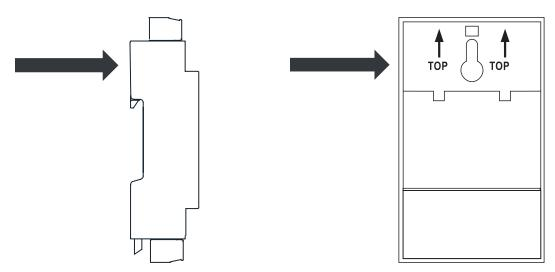
**Installation:** The device is provided with a hole for wall-mounting. Install the device after having prepared the dowel and relative screw on the wall.
