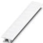
Marker for terminal blocks, Strip, white, labeled, can be labeled with: CMS-P1-PLOTTER, Horizontal: L1, L2, L3, N, PE, L1, L2, L3, N, PE, mounting type: snap into tall marker groove, for terminal block width: 6.2 mm, lettering field size: 6.15 x 10.5 mm, Number of individual labels: 10
