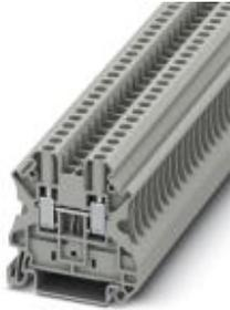
Feed-through terminal block, nom. voltage: 1000 V, nominal current: 32 A, connection method: Screw connection, number of connections: 2, cross section: 0.14 mm<sup>2</sup> - 6 mm<sup>2</sup>, AWG: 26 - 10, width: 6.2 mm, height: 46.9 mm, color: gray, mounting type: NS 35/7,5, NS 35/15
