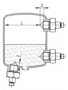
The apex should protrude into the container
